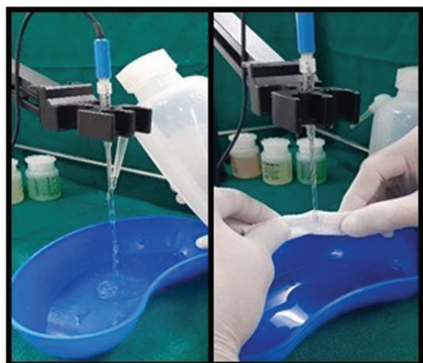
Figure 4: Microelectrode being rinsed with distilled water and dabbed dried with tissue paper.
