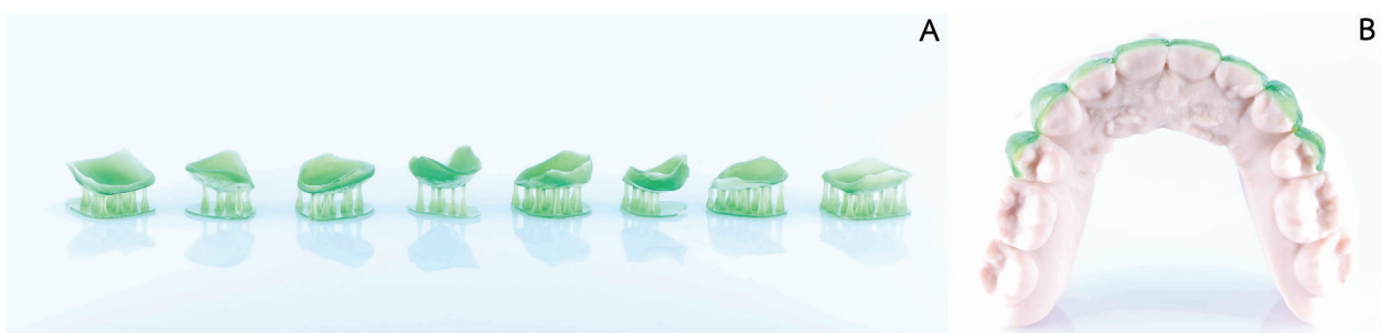
Figure 24: Castable resin from 3d printing.
