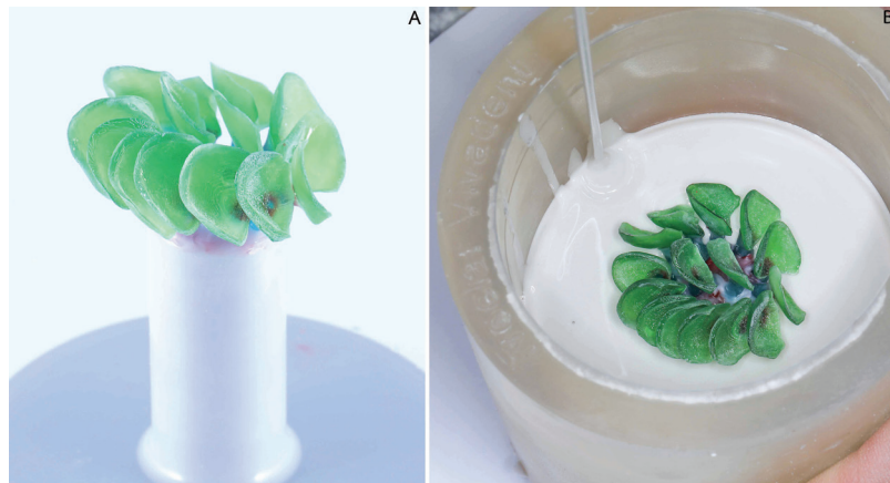
Figure 25: Representative: (A) The castable resin spruing on investment ring. (B) Pouring investment.
