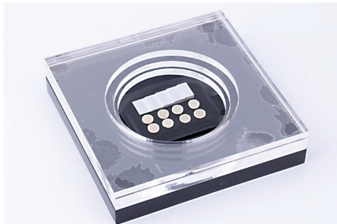
Figure 4: Clear acrylic hallow platform which covered the specimens and aluminium step wedge.
